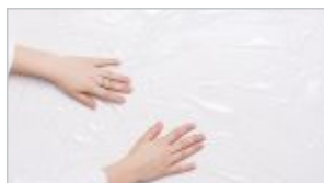
phase III: Apply strips of stretch foil upon wet material and slightly form the pattern with a hand.
