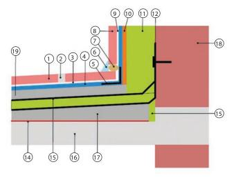
Fig. 2. Isolation expansion joint in terrace surface over a heated room – top layer of ceramic tiles
