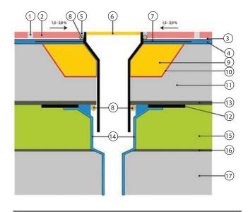
Fig. 3 Mounting and sealing a point floor inlet in a terrace slab over a heated room – top layer of ceramic tiles.
