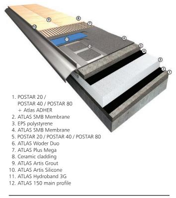
Photo 1. Terrace layers arrangement, option A.
