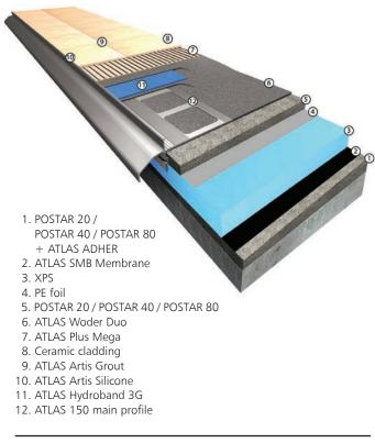
Photo 2. Terrace layers arrangement, option B.
