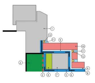
Fig. 5. Sealing the door frame threshold on a terrace or a balcony
