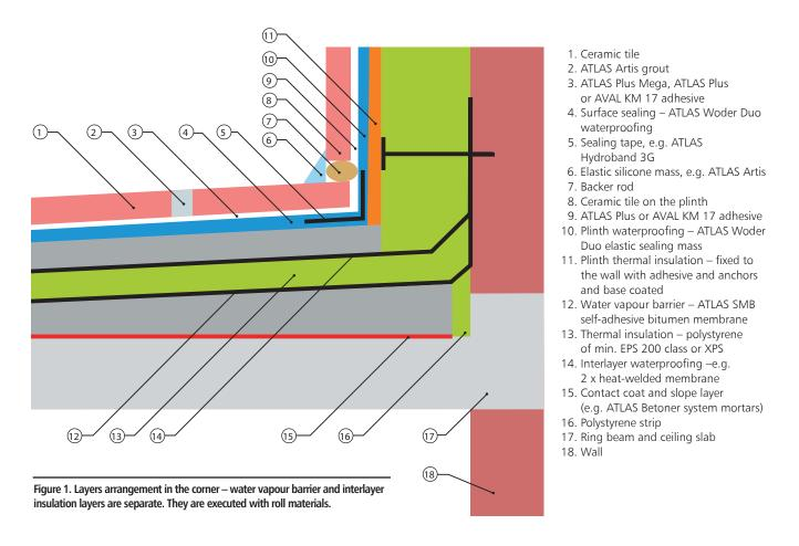
The slope layer must always be executed on the contact coat. For mortars from Postar line it is formed by ATLAS Adher mortar, or alternatively: mixture of water, ATLAS Elastic Emulsion and dry mortar. The substrate surface must be wetted to the matt-wet state and then the contact coat material rubbed into the substrate with a brush or a paintbrush. The slope layer is applied with "wet on wet" method (when the contact coat still makes fingers dirty).
