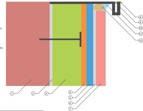
Figure 2. Set back of the plinth prevents from soaking by rainwater
