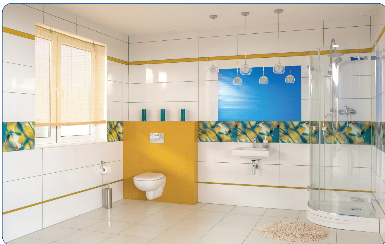
Photo 1. Selection of joints with a view to the colour depends on the functional issues. At the stage of colour matching it is recommended to keep in mind the place of installation. On the floors it is better to use darker tones, which are less likely to get dirty. In contrast, on the walls and decorative elements the colour of grouts may be lighter.
