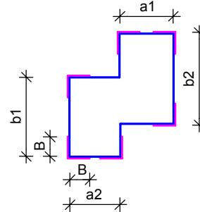
**No. 1.2.2 Arrangement of the panels and fixings for mineral wool - example**
