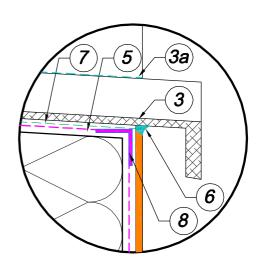
No. 1.3.4 Insulation of the under-reveal wall with the window frame even to the wall face with a corner profile
