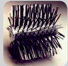
Manual machine and broom - devices once used for spotted render application.
