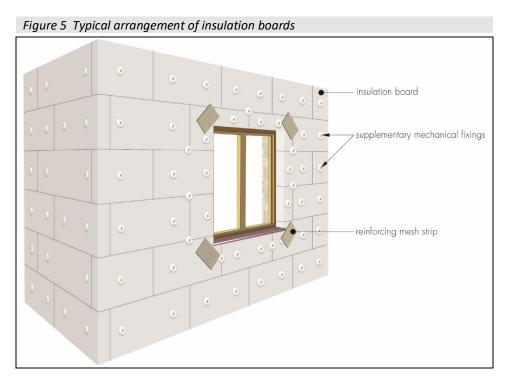
16.10 Prior to the application of the main reinforcing mesh, additional pieces of reinforcing mesh (approximate size 300 by 200 mm) should be used diagonally at the corners of openings and at window reveals (see Figure 5).
