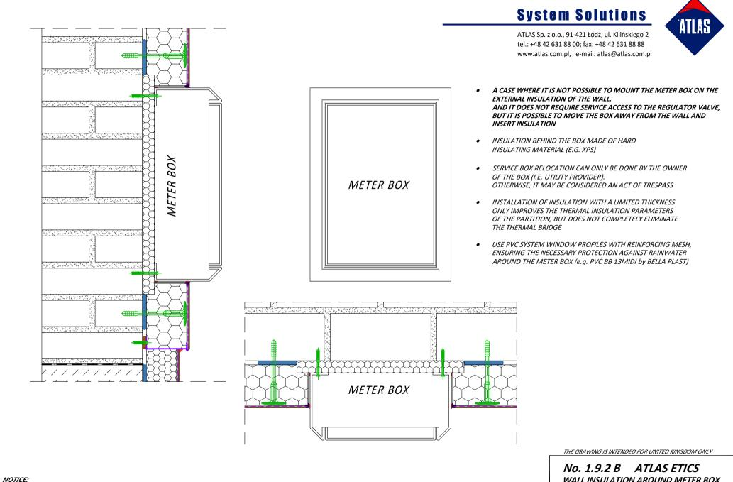
THE DETAILS PROVIDED ARE INFORMATIVE AND ARE TO HELP THE DESIGNER IN SELECTING THE PROPER SOLUTIONS. THEY ARE NOT EXHAUSTIVE AND HAVE TO BE ADAPTED BY THE DESIGNER TO THE INDIVIDUAL CIRCUMSTANCES APPROPRIATE TO THE SPECIFIC IMPLEMENTATION WALL INSULATION AROUND METER BOX
