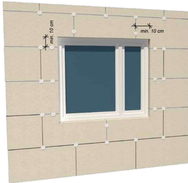
an example of correct arrangement of panels in the corners of windows
