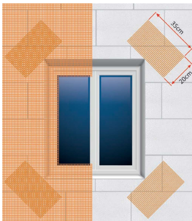
places for installing additional diagonal reinforcements
