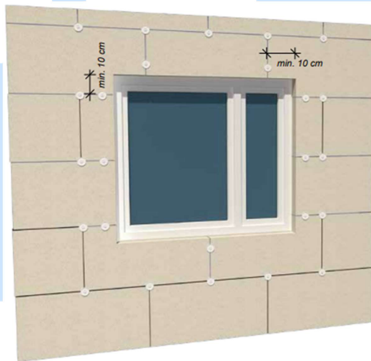
an example of correct arrangement of panels in the corners of windows
