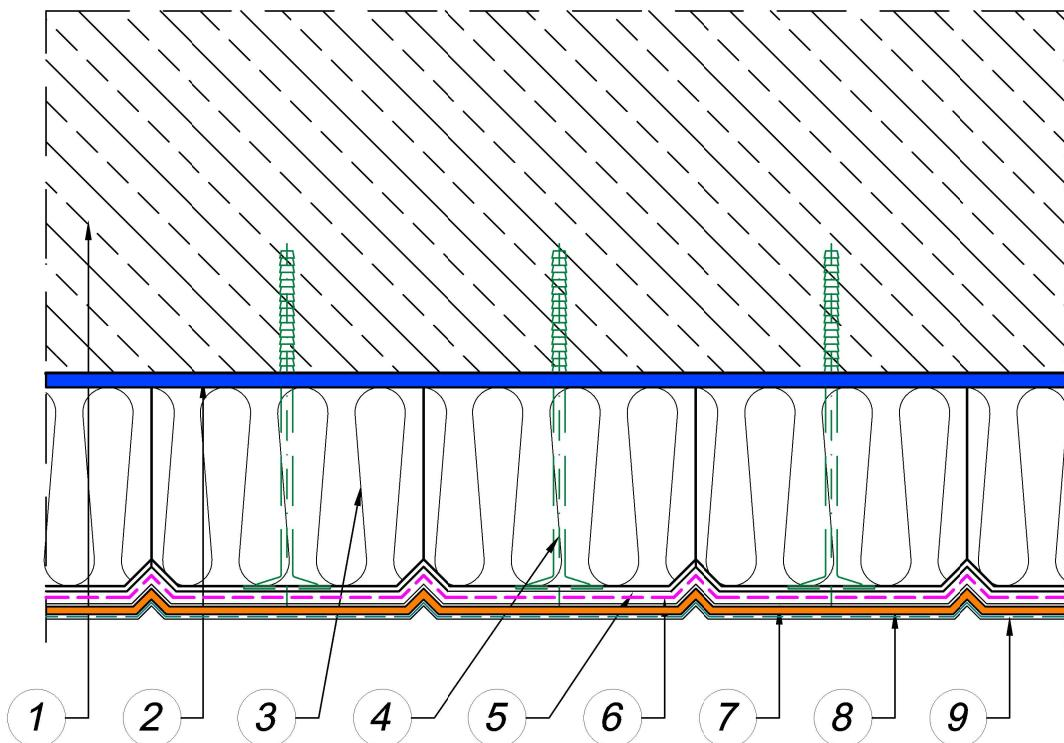
*Exemplary arrangement of ATLAS ROKER G system - type II***1. CEILING:**
